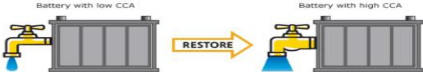
Figure 2: CCA is shown with free-flowing and restricted taps.
